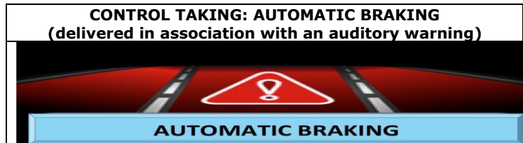
Figure 55: pictogram delivered by MOVIDA to inform the driver about the automatic “Emergency Braking”, when implemented by the AdCoS
