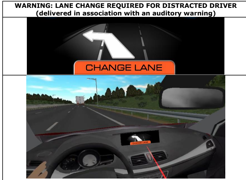
Figure 62: Visualization of MOVIDA outputs delivered to support the Lane Change manoeuvre of a visually distracted driver
