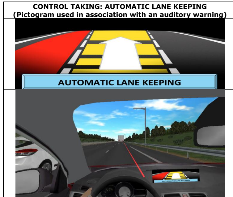
Figure 64: Visualization of MOVIDA outputs when the Automatic Lane Keeping function is activated
