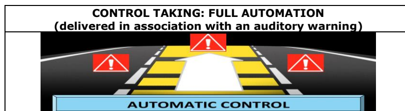
Figure 57: pictogram use by MOVIDA to inform the driver about the “Full Automation” status of the AdCoS (i.e. automatic Lane Keeping and Braking)
