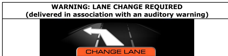
Figure 52: pictogram delivered by MOVIDA to warn a distracted driver that a Lane Change Manoeuvre is required and possible
