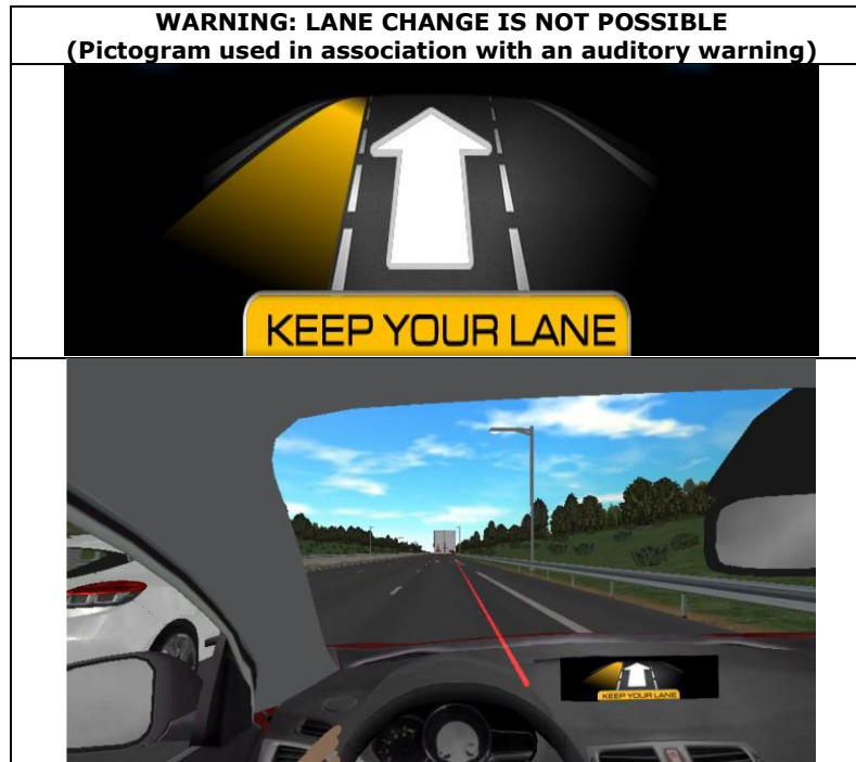
Figure 63: Visualization of MOVIDA outputs to warn the driver of a dangerous Lane Change manoeuvre
