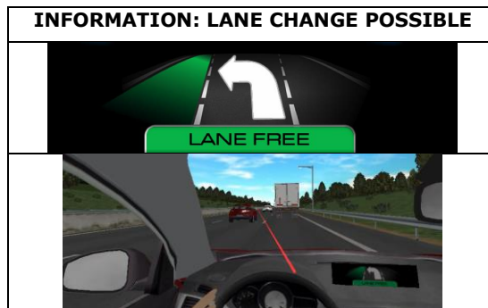
Figure 51: pictogram delivered by MOVIDA (on the in-vehicle display) to inform a non-distracted driver that the Lane Change Manoeuvre is possible
