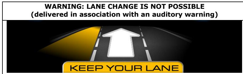
Figure 53: pictogram delivered by MOVIDA to warn the driver that that a Lane Change Manoeuvre is not possible
