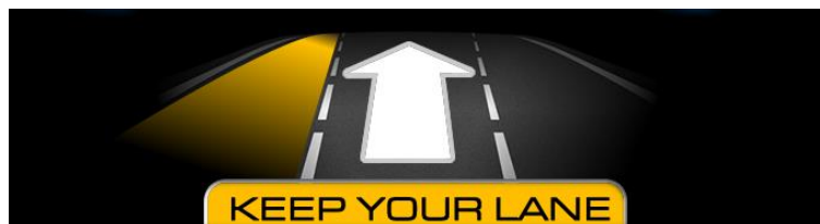
Figure 9: HMI to support the driver if s/he wants to change the lane but a car is approaching from behind
