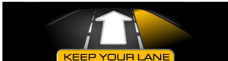
Figure 10: HMI to support the driver if s/he wants to re-enter the lane but a car is on the right lane
