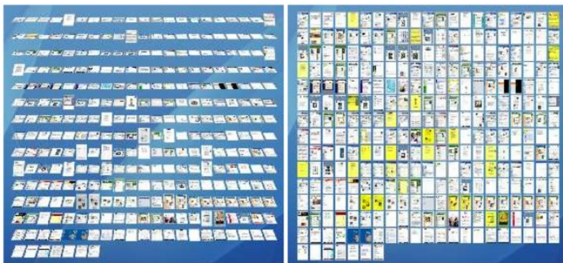
Figure 16: Left side: less important documents are tilted away from the user. Right side: effect of colour and intensity is used
