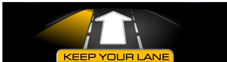
Figure 8: HMI to support the driver if s/he wants to change the lane but a car is approaching from behind
