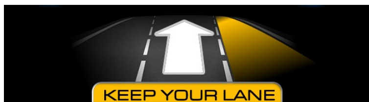
Figure 9: HMI to support the driver if s/he wants to re-enter the lane but a car is on the right lane
