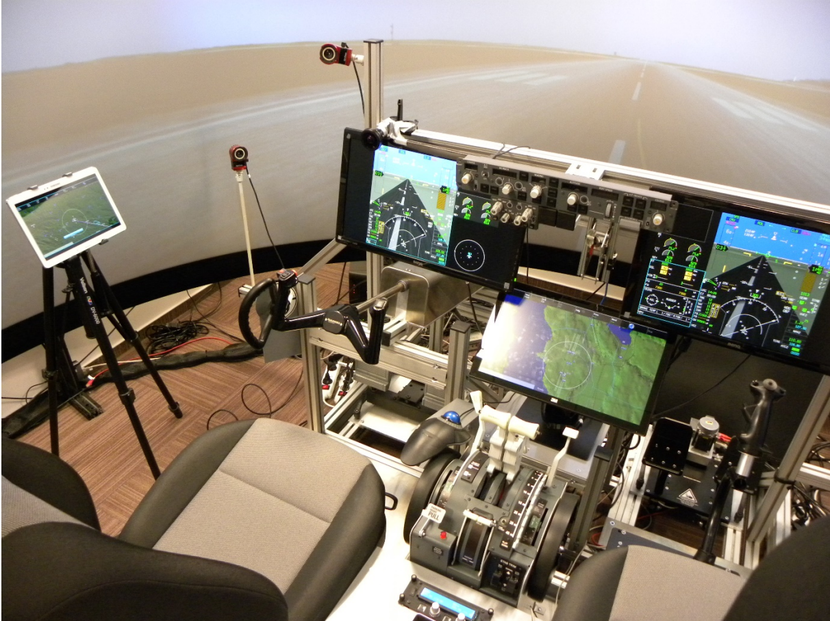
Figure 10: Aeronautic simulator with the cameras tracking the pose and detecting the implicit gestures.
