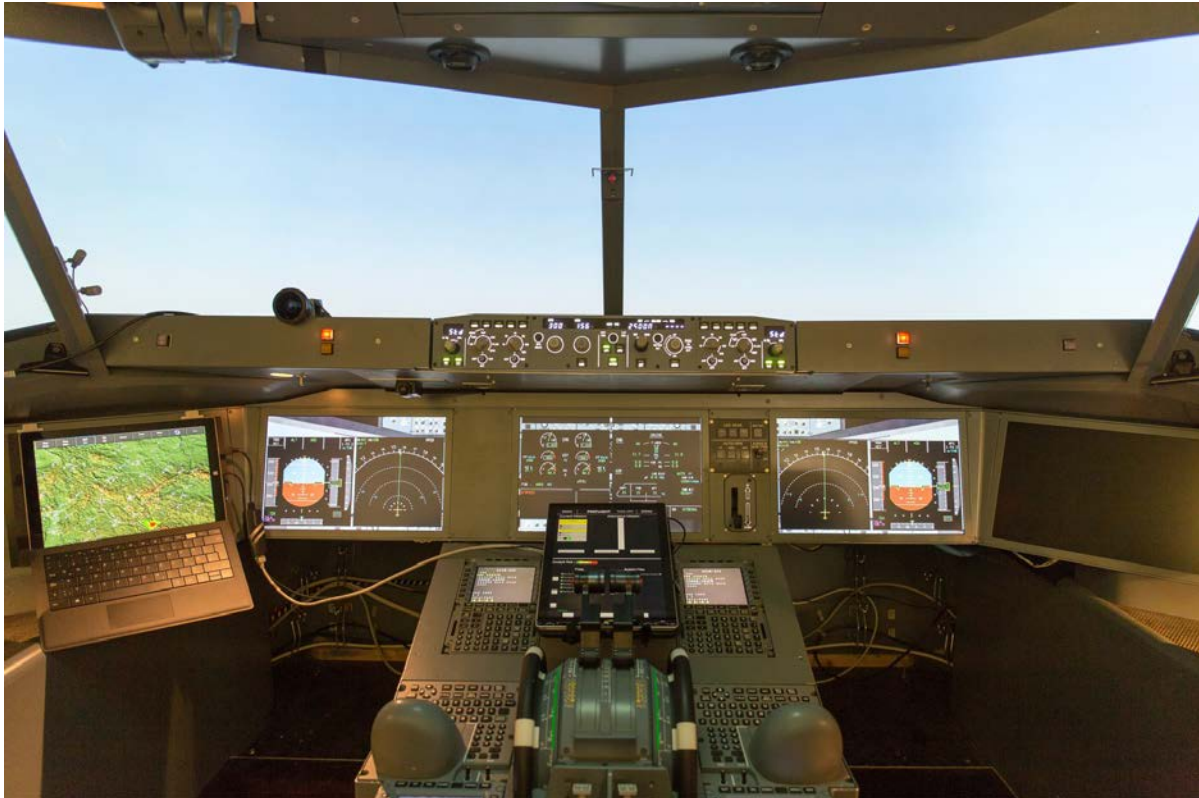
Figure 13: Aeronautic simulator with the gaze estimation camera (placed on the lower edge of the windshield).
