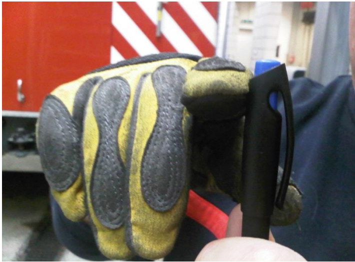
Figure 4: Working glove: harder, smaller fingertip.
