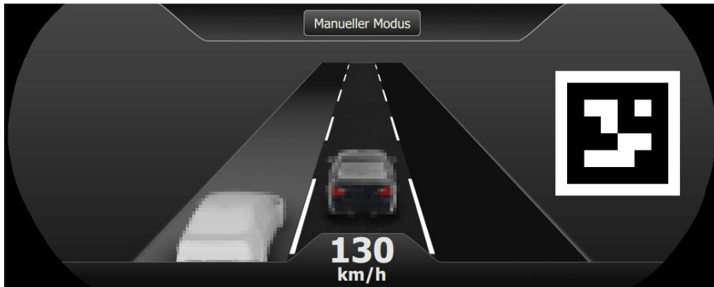
Figure 36: Instrument cluster of the HMI in manual mode with eye-tracking marker with approaching car from behind without driver intention to overtake.
