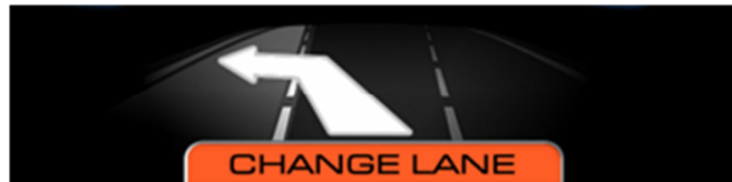
Figure 47: pictogram delivered by MOVIDA to warn a distracted driver that a Lane Change Manoeuvre is required and possible.
