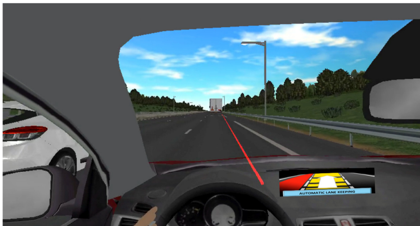
Figure 73: Visualization of MOVIDA outputs when the Automatic Lane Keeping function is activated
