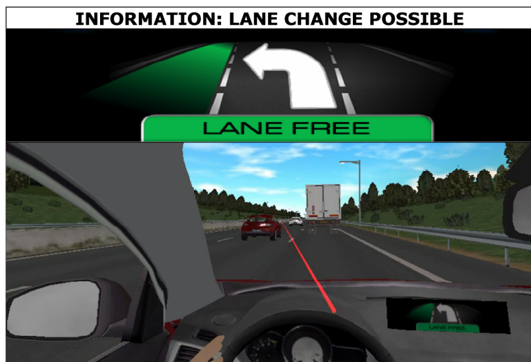
Figure 46: pictogram delivered by MOVIDA (on the in-vehicle display) to inform a non-distracted driver that the Lane Change is possible.
