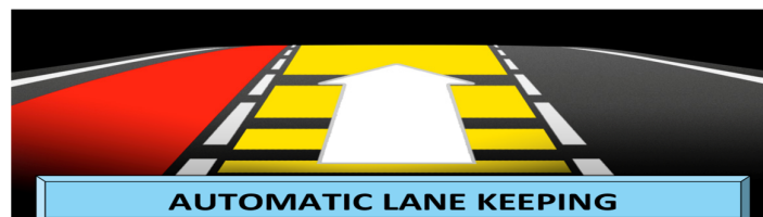
Figure 51: pictogram delivered by MOVIDA to inform the driver about the “Lane Keeping” automatic manoeuvre, when implemented by the AdCoS.
