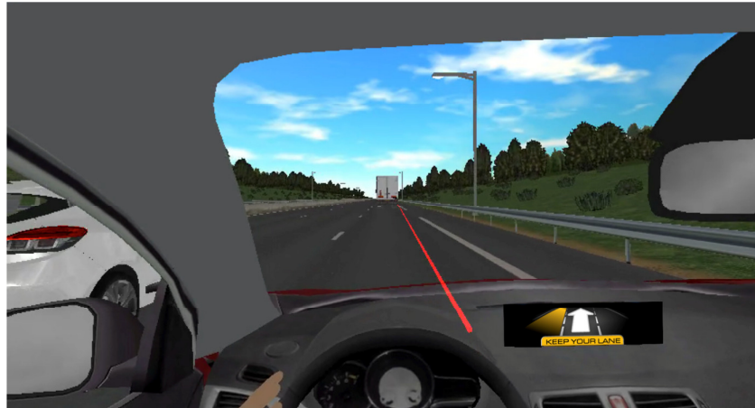
Figure 72: Visualization of MOVIDA outputs to warn the driver of a dangerous Lane Change manoeuvre
