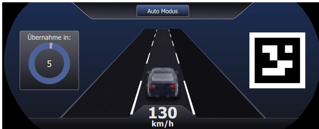
Figure 39: Instrument cluster of the HMI in automatic mode with eye-tracking marker and take-over request (“Übernahme in”) with remaining seconds.
