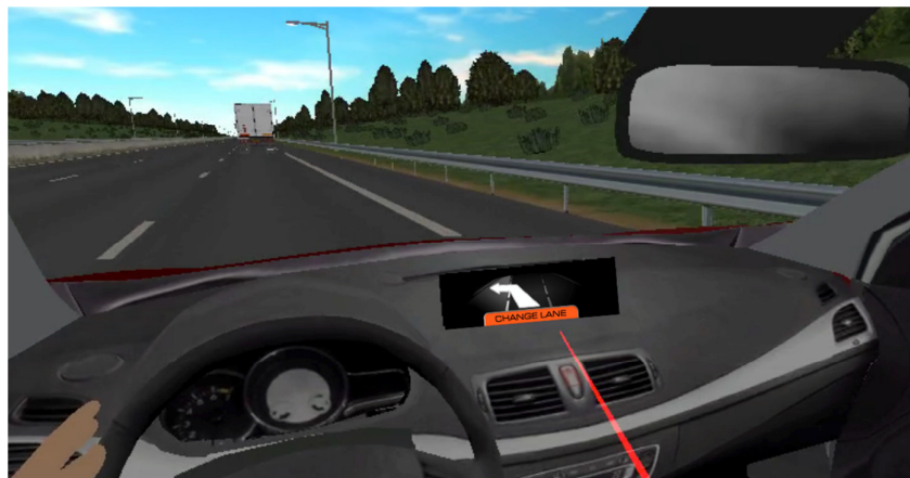
Figure 71: Visualization of MOVIDA outputs delivered to support the Lane Change manoeuvre of a visually distracted driver
