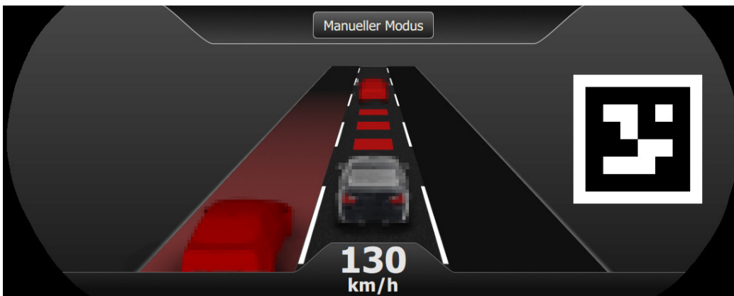
Figure 37: Instrument cluster of the HMI in manual mode with eye-tracking marker and critical distance to car in front and approaching car from behind with overtaking intention of the ego vehicle.
