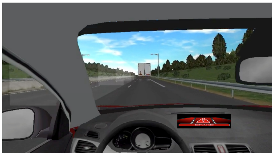
Figure 58: MOVIDA warning to alert a distracted driver of a Frontal Collision risk (delivered in association with an Auditory warning).
