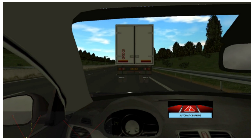
Figure 75: Visualization of MOVIDA outputs when the Automatic Braking is implemented by the AdCoS
