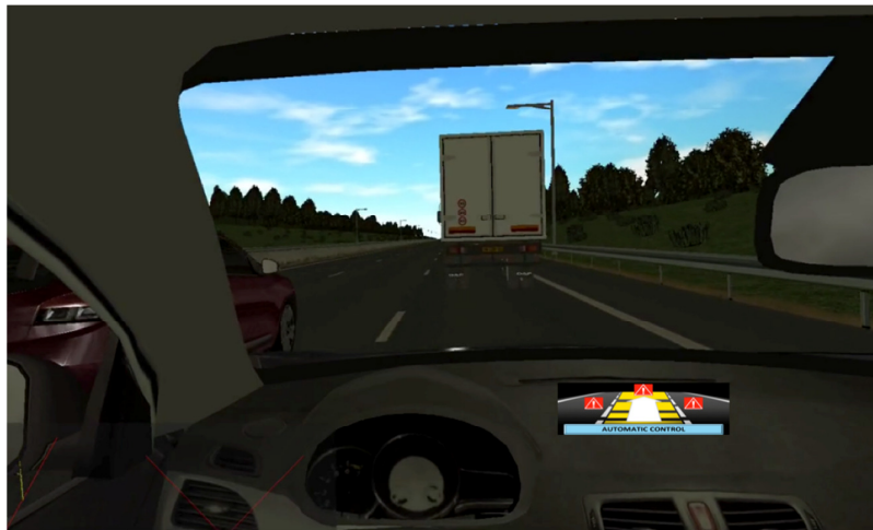
Figure 76: Visualization of MOVIDA outputs when the Automatic Lane Keeping and Braking functions are jointly implemented
