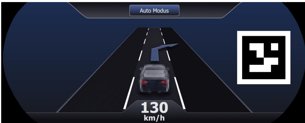
Figure 38: Instrument cluster of the HMI in automatic mode with eye-tracking marker and lane-change information provided to the driver.
