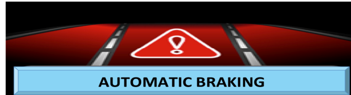
Figure 50: pictogram delivered by MOVIDA to inform the driver about the automatic “Emergency Braking”, when implemented by the AdCoS.
