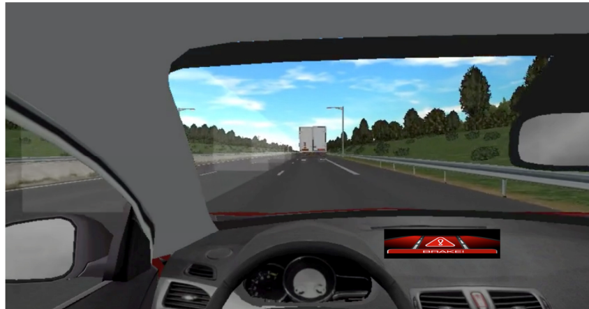
Figure 74: MOVIDA outputs to warn the driver of frontal collision risk
