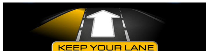
Figure 48: pictogram delivered by MOVIDA to warn the driver that that a Lane Change Manoeuvre is not possible.
