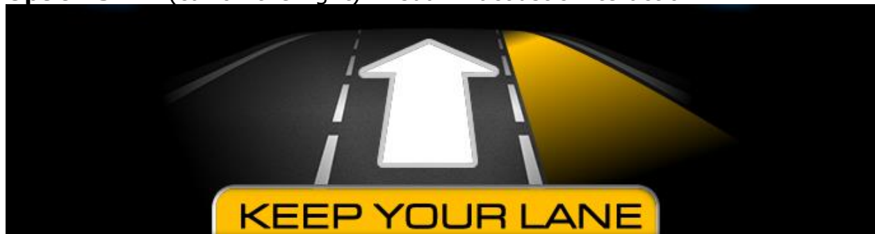
Figure 32: HMI to support the driver while re-entering into the original lane (task 3).
