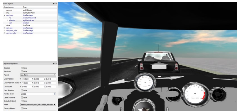
Figure 6: Pro-SiVIC simulation with COSMODRIVE at the wheel
