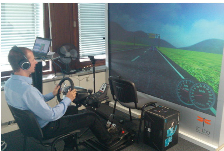
Figure 8. The TWT driving simulator, used for experiments to assess features correlating with the cognitive distraction degree of the driver.
