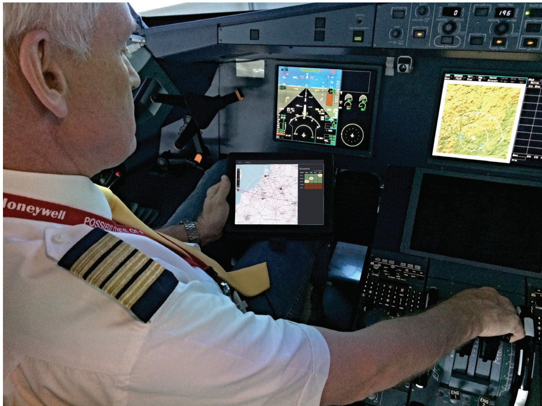
Figure 20. Diversion assistant provides guidance for selecting an alternate airport based on analysis of up-to-date information
