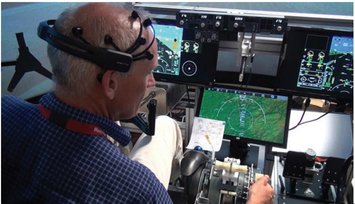
Figure 23: Application of physiological signals such as EEG was demonstrated in the cockpit as capable to monitor pilot's workload
